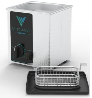
The **U100H** is a 1.5Litre ultrasonic bath with heating function to reduce processing time. Each **U-Series** is supplied complete with a stainless steel basket and ABS plastic lid, useable as a drip tray to collect excess water when the basket is removed from the tank.
