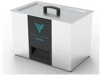
The Qi-400 is a 30Litre ultrasonic cleaner with a menu driven, LCD control panel. This allows simple adjustment of cycle time (0 to 99mins or infinity mode), temperature (ambient to 80°C), ultrasonic power and frequency mode for precise and accurate processing.
