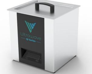
The Qi-300 is a 17Litre ultrasonic cleaner with a menu driven, LCD control panel. This allows simple adjustment of cycle time (0 to 99mins or infinity mode), temperature (ambient to 80°C), ultrasonic power and frequency mode for precise and accurate processing.
